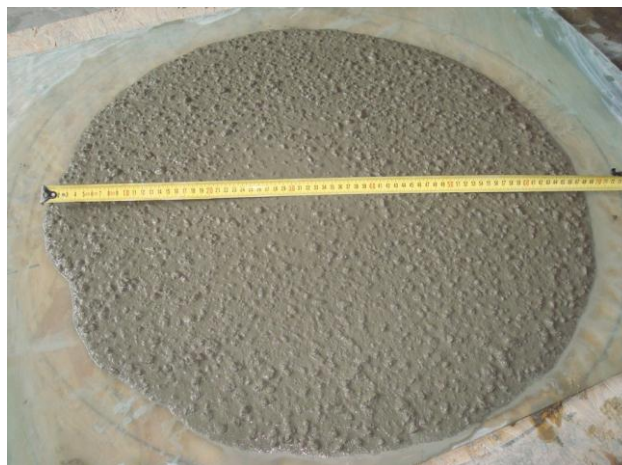
Figure 7. Flow test of the mixture 4.
