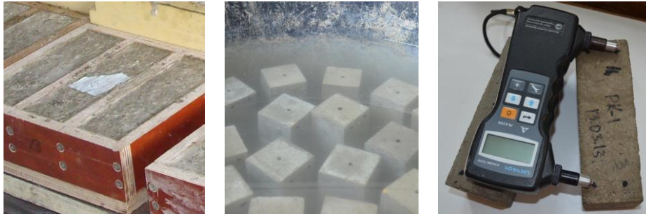
Figure 4. Produced prismatic shape concrete specimens for frost resistance test.
