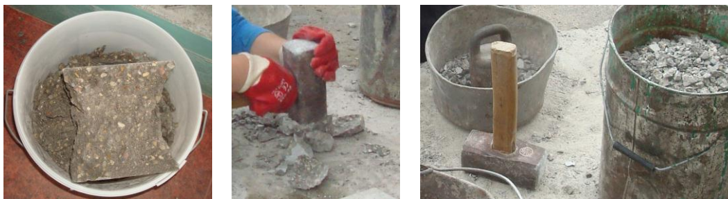
Figure 2. The manual obtaining process of recycled concrete aggregates.
