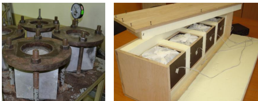
Figure 3. Equipment to measure permeability (left) and hydration temperature inside of concrete mixtures (right).
