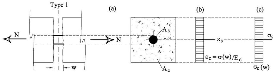
Figure 3. RC ties: (a) Geometrical properties of Type 1 cross-section; (b) State of strain; (c) State of stress.
