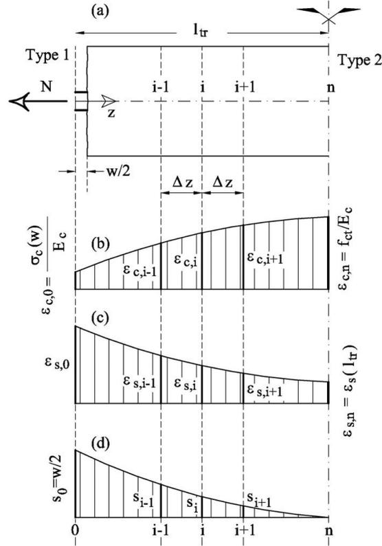
Figure 6. The portion of a RC tie used to model the tension stiffening.
