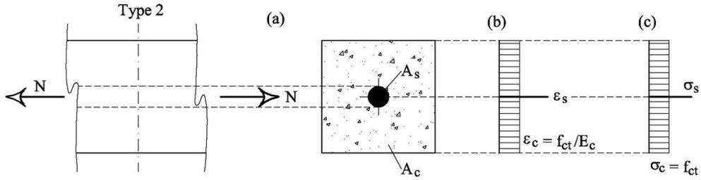
Figure 4. RC ties: (a) Geometrical properties of Type 2 cross-section; (b) State of strain; (c) State of stress.
