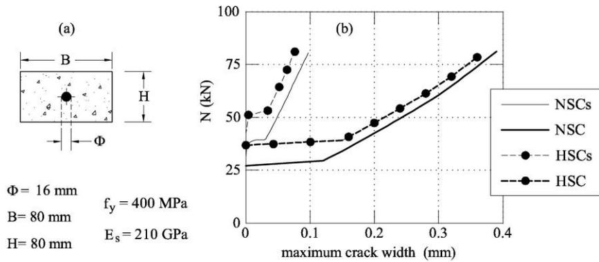
Figure 8. Application of the proposed tension stiffening model: (a) geometry of the RC ties; (b) predicted crack width.
