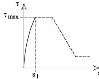
Figure 5. Bond-slip relationships for plain (fib, 2010) and fiber-reinforced concrete (Harajli 1995).
