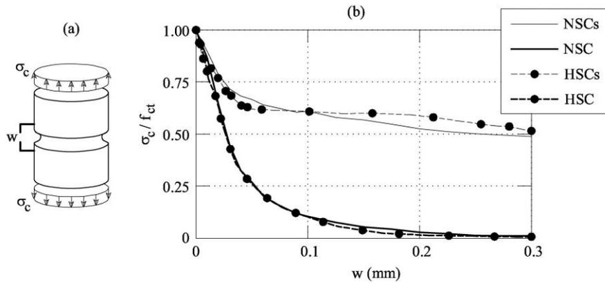
Figure 1. Uniaxial tensile tests performed by Noghabai (1998): (a) notched specimen; (b) normalised stress vs. crack opening displacement curves.
