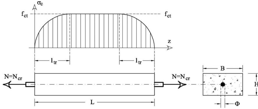
Figure 2. Tensile stresses in the concrete surrounding a steel reinforcing bar in tension.
