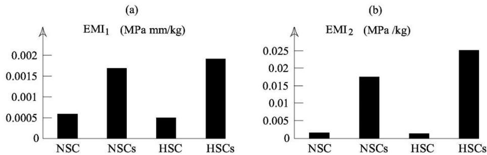
Figure 9. Eco-Mechanical Index: (a) values of  $EMI_1$  ; (b) values of  $EMI_2$ .
