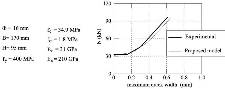
Figure 7. Comparison between the maximum crack width predicted by the proposed model and the values measured by Mitchell et al. (1996).
