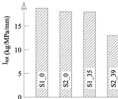
Figure 5 – Evaluation of the global eco-mechanical index  $I_{tot}$  for the SCC investigated in this project.
