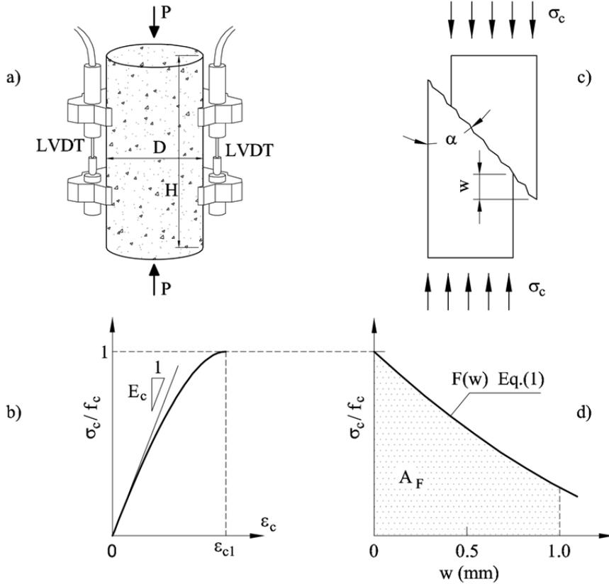
Figure 1 – Uniaxial compressive tests on SCC cylinders: a) geometrical properties and position of the LVDTs; b) pre-peak stress-strain curve; c) the kinematic variables involved in the softening branch; d) post-peak response in terms of  $F(w)$  (i.e. relative cohesive stress vs. inelastic shortening  $w$ ).
