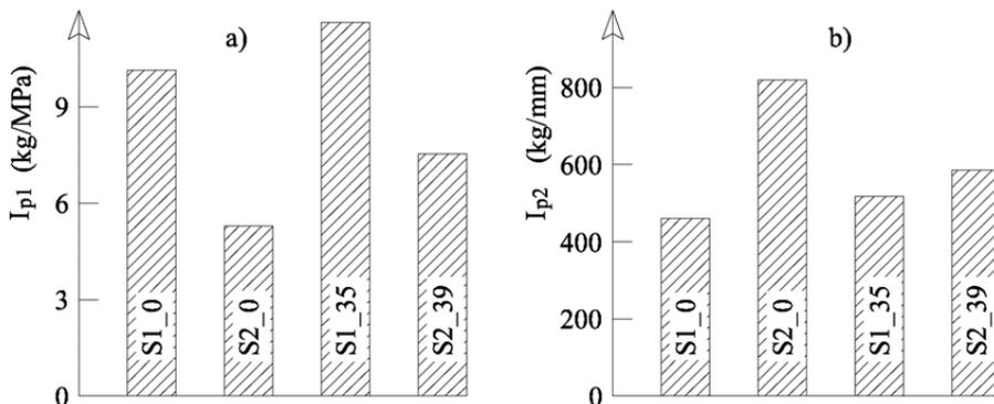
Figure 4 – Eco-mechanical indexes introduced for the SCC and FR-SCC investigated in this project: a)  $I_{p1}$  indexes of the pre-peak stage; b)  $I_{p2}$  indexes of the post-peak stage.
