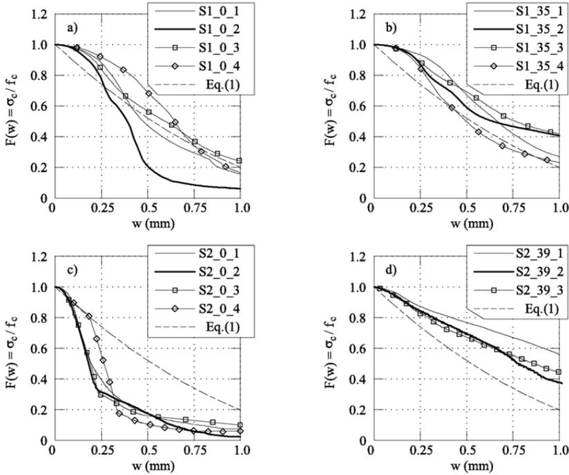
Figure 3 - The  $F(w)$  curves resulting from tests: a) plain SCC of Series 1; b) Series 1 with  $35 \text{ kg/m}^3$  of steel fibers; c) plain SCC of Series 2; b) Series 2 with  $39 \text{ kg/m}^3$  of steel fibers.
