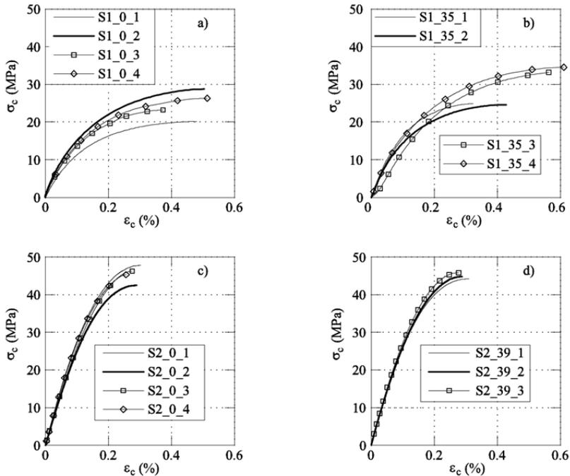
Figure 2 - The  $\sigma_c$ - $\varepsilon_c$  curves resulting from tests: a) plain SCC of Series 1; b) Series 1 with 35 kg/m<sup>3</sup> of steel fibers; c) plain SCC of Series 2; b) Series 2 with 39 kg/m<sup>3</sup> of steel fibers.
