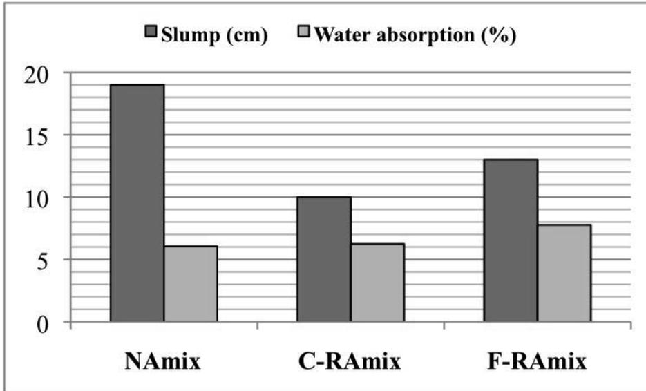
Figure 2 - Physical properties of concrete mixes.
