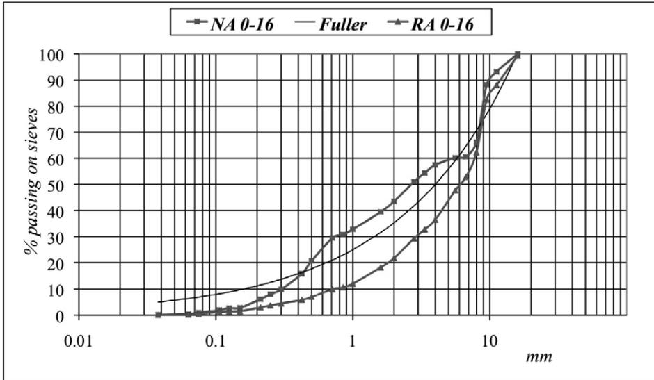
Figure 1 - Grain size distribution of recycled aggregates (RA<sub>0-16</sub>) and natural aggregates (NA<sub>0-16</sub>), compared with Fuller distribution ( $D_{max} = 16$  mm).
