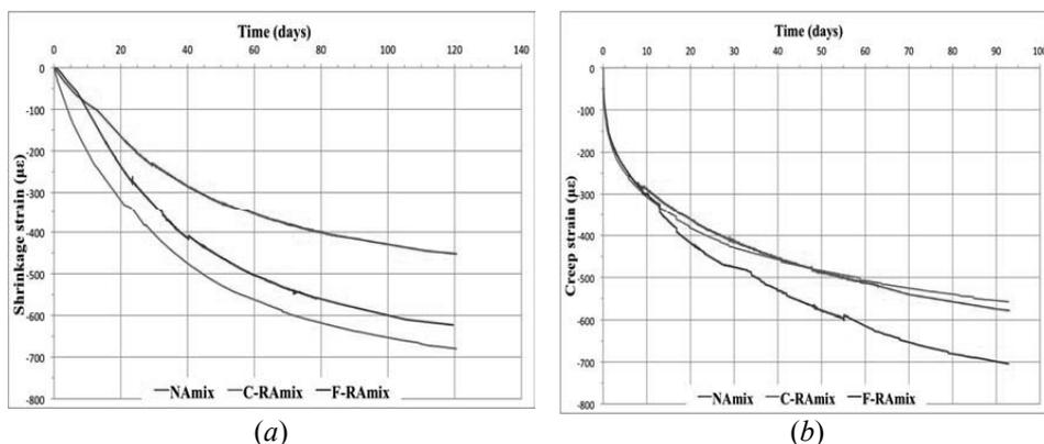
Figure 4 - Shrinkage strains (a) and creep strains (b) of the investigated concrete mixes.
