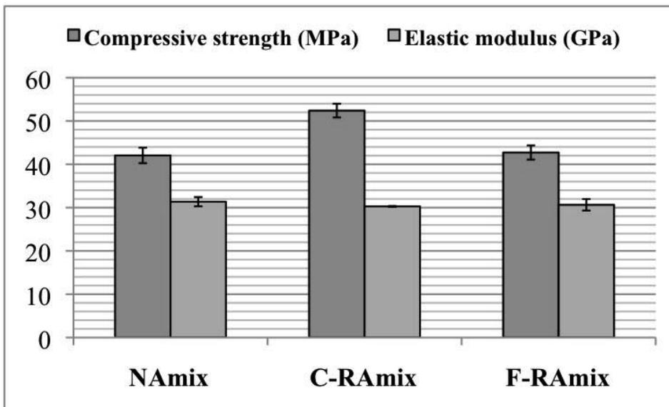
Figure 3 - Mechanical properties of the concrete mixes.
