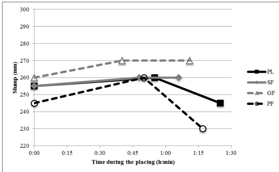
Figure 3. Slump vs. time.
