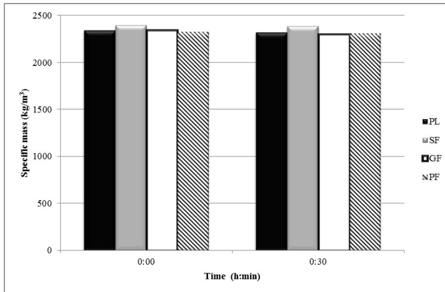
Figure 2. Specific mass of fresh concrete vs. time.
