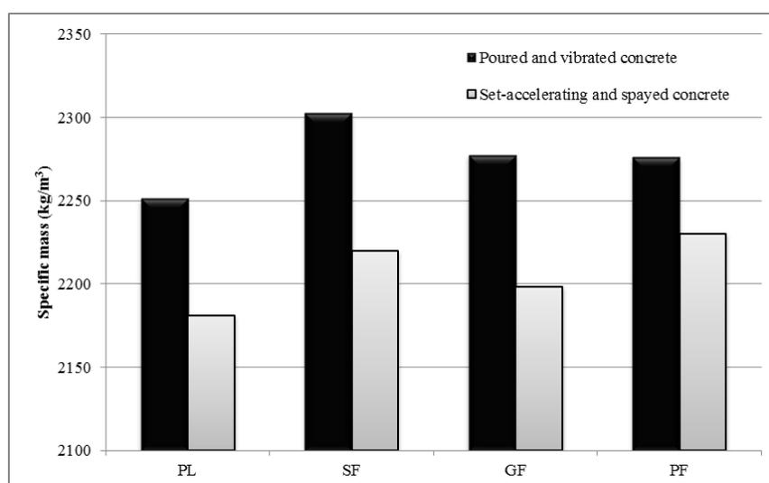
Figure 5. Specific mass of hardened concretes and shotcretes after 28 days.
