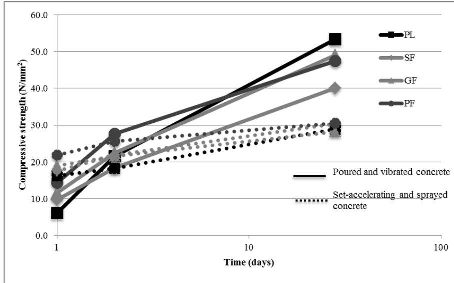
Figure 6. Compressive strength vs. time for specimens with and without set-accelerating admixture.
