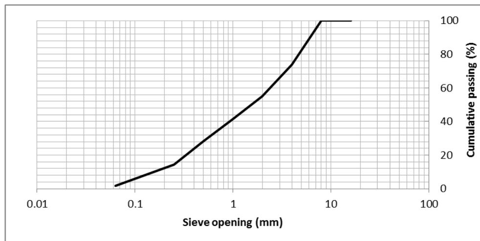
Figure 1. Combined aggregate grading.
