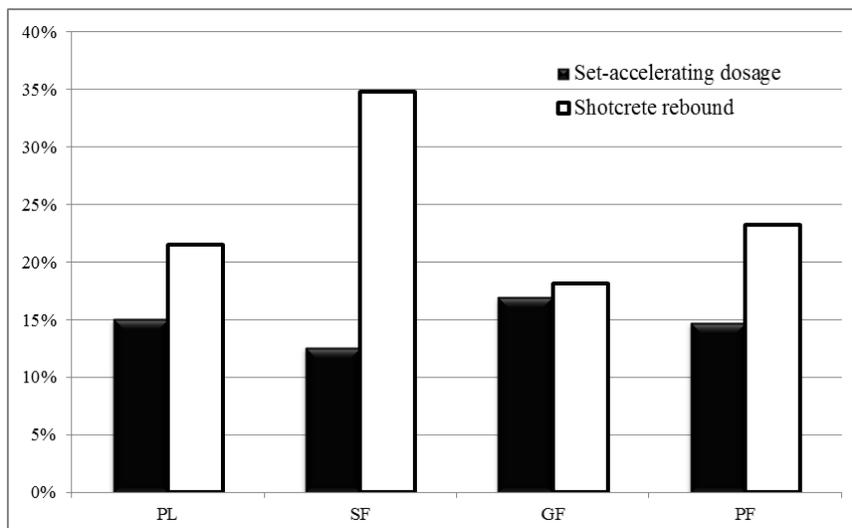
Figure 4. Set-accelerating admixture dosage and shotcrete rebound.
