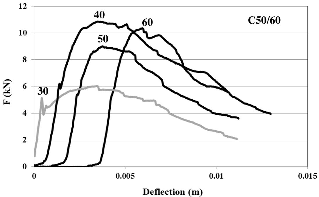
Figure 4. Force vs. deflection curve under flexural stress for C50/60 FRC. Numbers on curves indicate the fibers dosage ( $\text{kg/m}^3$ ).
