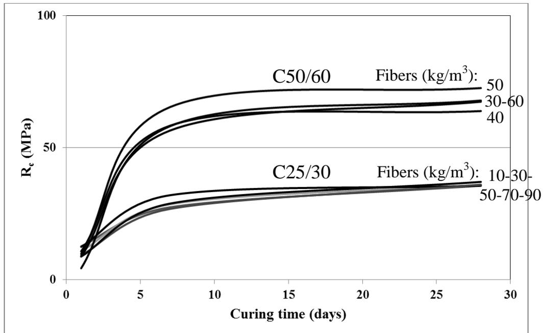
Figure 1. Strength development with curing time of the different FRCs.
