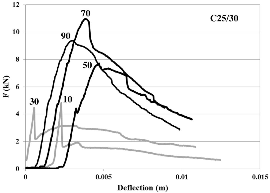
Figure 3. Force vs. deflection curve under flexural stress for C25/30 FRC. Numbers on curves indicate the fibers dosage ( $\text{kg/m}^3$ ).
