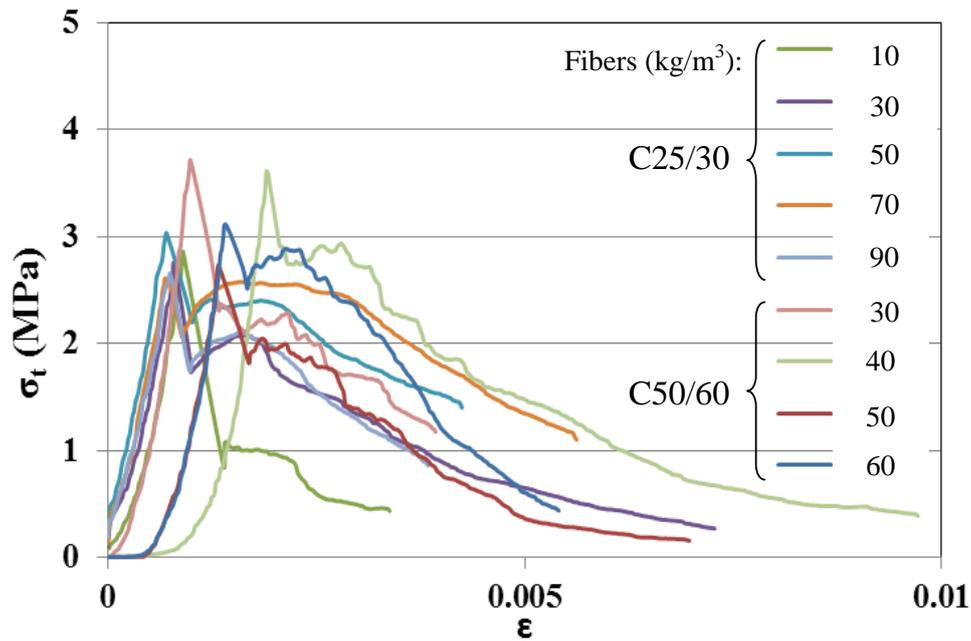
Figure 2. Stress-strain curves under splitting tension of the different FRCs.
