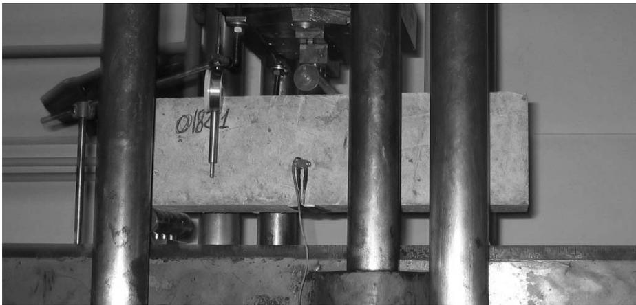
Figure 3 - Beam under third-point loading: test setup.
