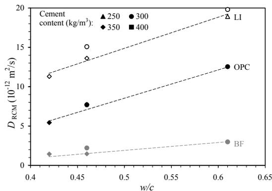
Figure 7 - Chloride diffusion coefficient  $D_{RCM}$ , as average of 2 concrete specimens cured 28 days, depending on the water/cement ratio, the type of cement (Portland cement, OPC, cement with 30% limestone, LI, 70% of cement with blast furnace slag, BF) and the dosage of cement (Bertolini et al. 2008).
