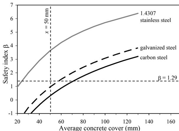
Figure 10 - Thickness of concrete cover required to ensure an average service life of 50 years for a reinforced concrete element exposed in the splash zone, depending on the index  $\beta$  and the type of reinforcement: carbon steel, galvanized steel, and type 1.4307 stainless steel (average annual temperature = 30°C, blast furnace slag cement with  $w/c$  ratio equal to 0.45) (Bertolini et al. 2010).
