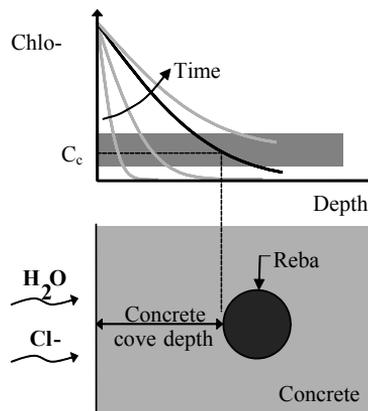
Figure 3 – Initiation of chloride induced corrosion and factors involved.
