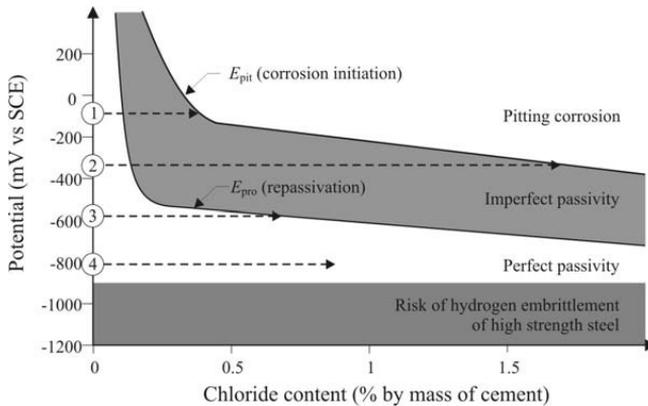
Figure 5 – Pedefferri Diagram, showing the effect of steel potential on the chloride threshold level (adapted from Pedefferri, 1995). Different electrochemical conditions of steel are depicted: 1 = steel in concrete exposed to the atmosphere, 2 = steel subjected to cathodic prevention, 3 = steel subjected to cathodic protection, 4 = steel in submerged concrete.
