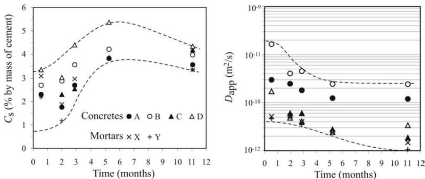
Figure 4 – Example of changes of  $C_s$  and  $D_{app}$  calculated by fitting chloride profiles measured on concrete specimens measured after different times of exposure to wetting/drying cycles with 3.5% NaCl solution. A: portland cement,  $w/c = 0.5$ , B: portland cement,  $w/c = 0.65$ , C: slag cement,  $w/c = 0.5$ , D: slag cement,  $w/c = 0.65$ , X: pozzolanic cement,  $w/c = 0.4$  (repair mortar); Y: proprietary repair mortar (Bertolini et al., 2002).
