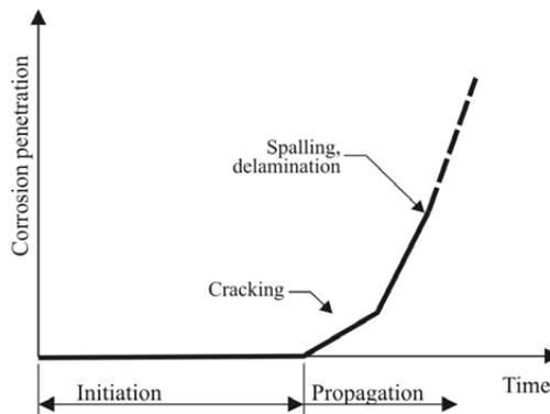
Figure 2 – Example of evolution in time of corrosion-related effects in reinforced concrete structures (adaptation of Tuutti's diagram).
