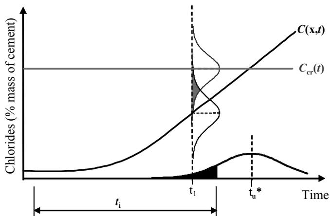
Figure 6 - Example of a probabilistic approach for the evaluation of service life for a structure subject to chloride-induced corrosion.
