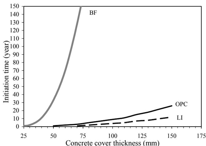
Figure 9 – Time of initiation of corrosion calculated for a safety index of 1.29 as a function of the thickness of concrete cover and the type of binder ( $w/c$  ratio 0.45, average annual temperature = 20°C) (Bertolini et al. 2010).
