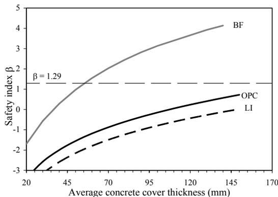
Figure 8 - Thickness of concrete cover required to ensure an average service life of 50 years for a reinforced concrete element exposed in the splash zone, depending on  $\beta$  index and the type of binder ( $w/c$  ratio 0.45 and average annual temperature = 20°C) (Bertolini et al. 2010).
