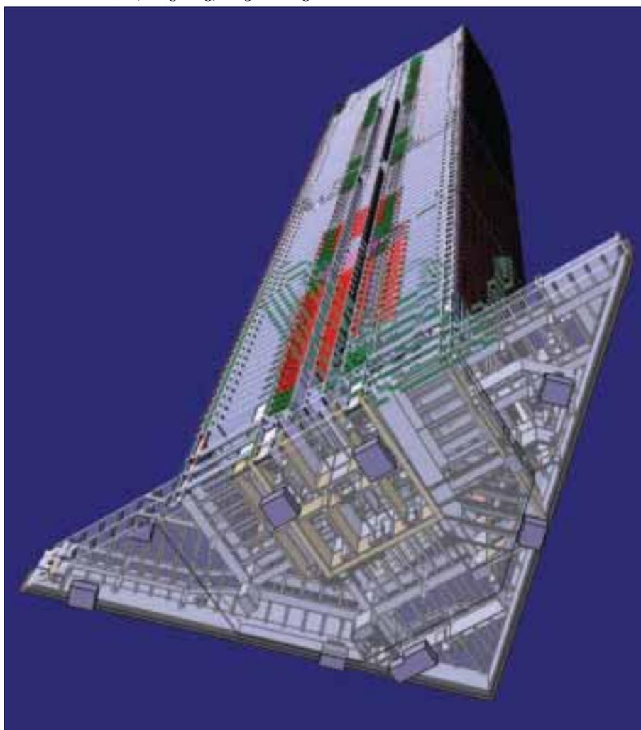
Simpler versions of the central model, such as centralised database modelling, are already being used. For example, the architect's extruded shape geometry can be fused with the engineer's analytical centreline geometry with scripted links for software interoperability, facilitating the comprehensive inclusion of design changes on a single parametric platform.
