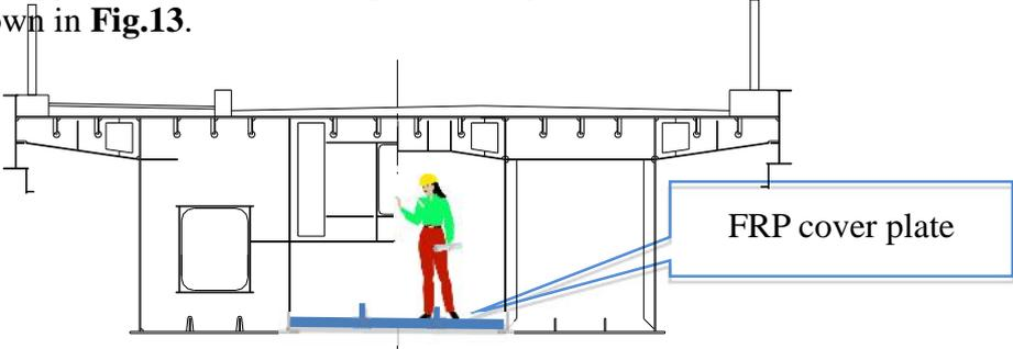
(a) Bridge cross section closed by FRP cover plate
