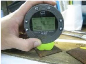
**Figure 3. Thickness gage.**
