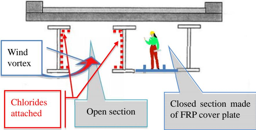
Figure 12. Smart usage of FRP cover plate for bridge maintenance
