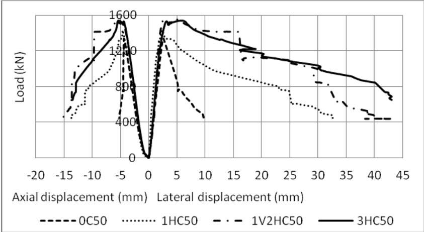
**Figure 3. Load-displacement curves for columns tested under 50 mm eccentricity.**
