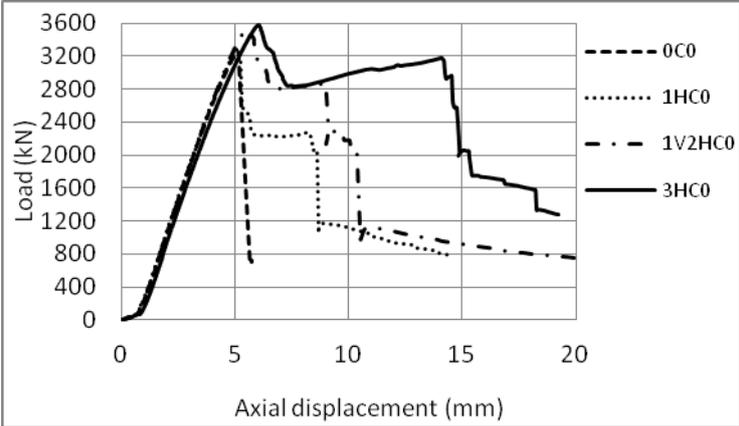
Figure 1. Load-displacement curves for columns tested under concentric loading.
