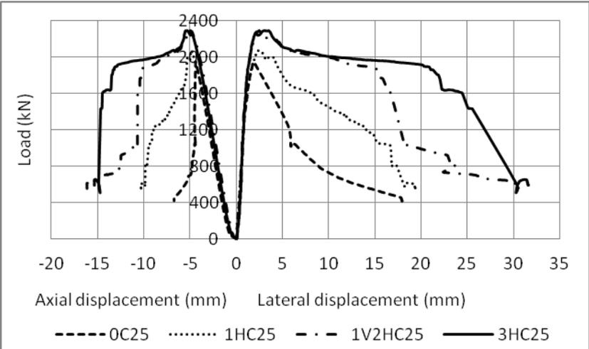
Figure 2. Load-displacement curves for columns tested under 25 mm eccentricity.
