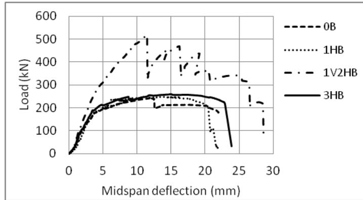
**Figure 4. Load-midspan deflection curves of beams tested under flexural loading.**
