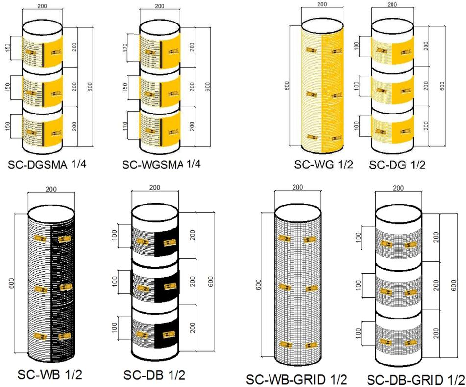
**Figure 1. Geometry of masonry columns and strengthening schemes - distances in (mm)**
