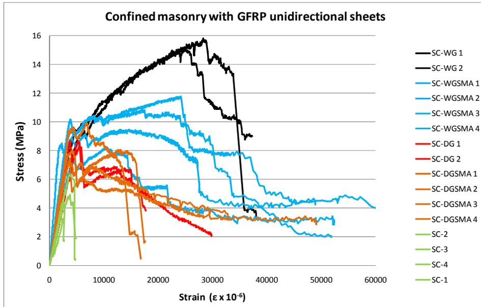
Figure 1. Experimental stress-strain curves for GFRP-confined masonry
