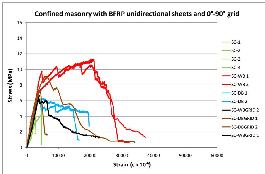
Figure 2. Experimental stress-strain curves for BFRP-confined masonry
